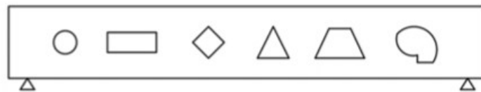
Figure 1. Various web openings shapes [1].
